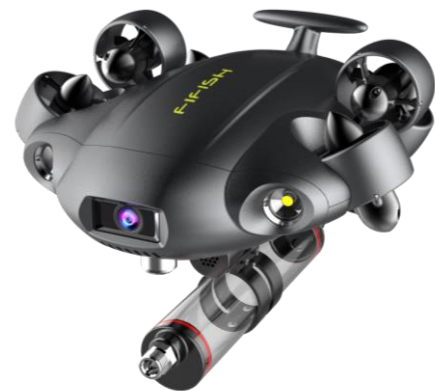
Water Sampler (500 mL) Collect water sample from certain depth and position
